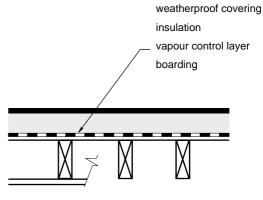
joists ceiling optional (d) Flat roof structure of timber or metal framed construction overlaid with a board decking at least 19 mm thick.
