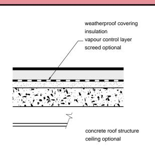
**(b)** Flat roof structure of in-situ or precast concrete with or without a screed.
