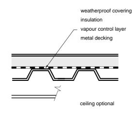
(f) Flat roof structure of timber or metal framed construction overlaid with a profiled metal decking.
