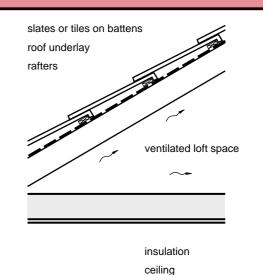
**(b)** Pitched roof structure of timber or metal framed construction.
