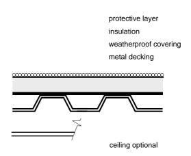
Note – These flat roof provisions do not apply to sheet metal weatherproof coverings such as lead, copper, zinc, etc. which require joints to allow for thermal movement.
